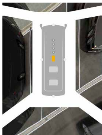
3_ The transmitted images are adjusted perspectively and consolidated to create a preview
